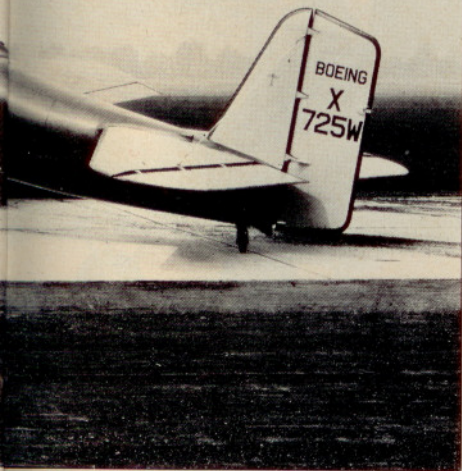
The first Boeing Monomail, Model 200. Note the three separate mail compartments ahead of the cockpit, the transition from a circular fuselage cross section forward to a vertical knife edge aft, and the large fillet between the wing and the fuselage.
